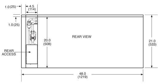
Notes: All Dimensions are in inches (mm). Optional autoflow valve, motorized water valve and disconnect box are shown.
