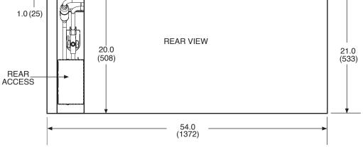
Notes: All Dimensions are in inches (mm). Optional autoflow valve, motorized water valve and disconnect box are shown.
