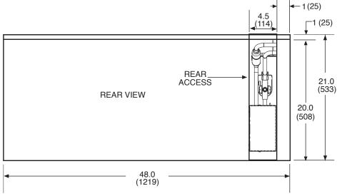
**Notes:** All Dimensions are in inches (mm) Optional autoflow valve, motorized water valve and disconnect box are shown.
