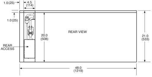
**Notes:** All Dimensions are in inches (mm). Optional autoflow valve, motorized water valve and disconnect box are shown.
