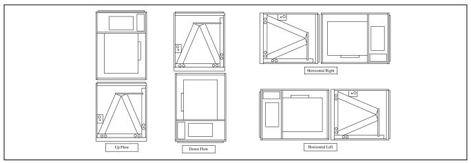
**Typical Applications with MC Multi-Position Coils**
