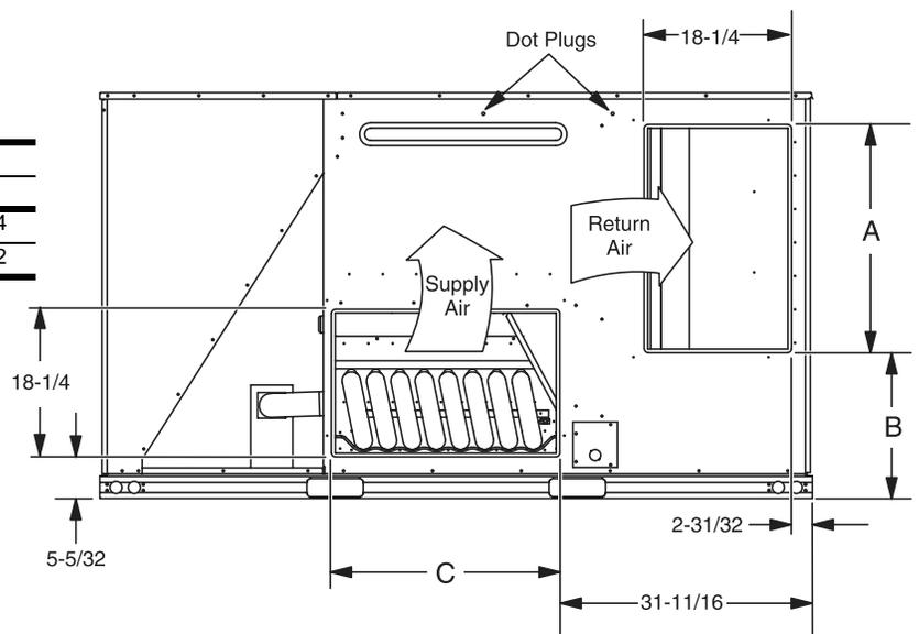
FIGURE 9 - REAR DUCT DIMENSIONS
