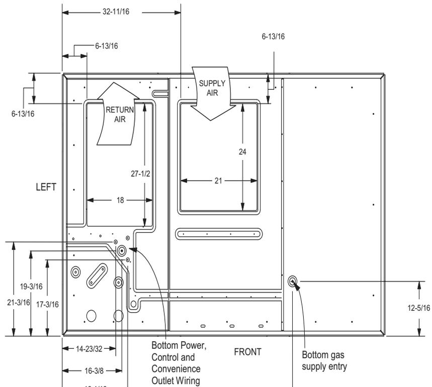
FIGURE 8 - BOTTOM DUCT OPENINGS (FROM ABOVE)
