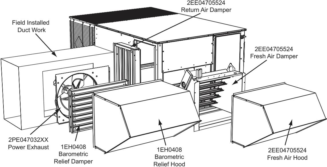
**FIGURE 13 - FIELD INSTALLED HORIZONTAL ECONOMIZER W/POWER EXHAUST**
